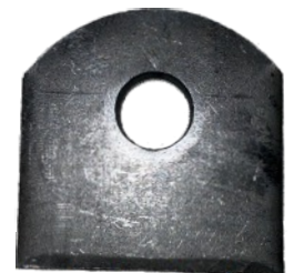
ORC7S Short "L" Rail Clip Placa Estillo "L" Corta 1" x 1-1/2" x 2" 3/8" hole, 9ga
